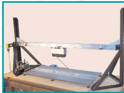
LASS (Laser-based Aggregate Scanning System) developed by ICAR Researchers
