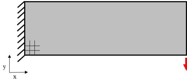
Figure 1: Cantilever beam example showing loading and boundary conditions.
