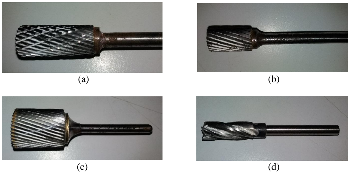
Figure 4 Different types of cutter available for EPS machining (a) Diamond deburring cutter, (b) Cylindrical deburring cutter, (c) Cylindrical flat end deburring cutter and (d) Flat end milling cutter
