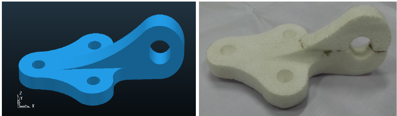
Figure 9 (a) CAD model of the bracket (b) Rapid Prototyped EPS pattern
