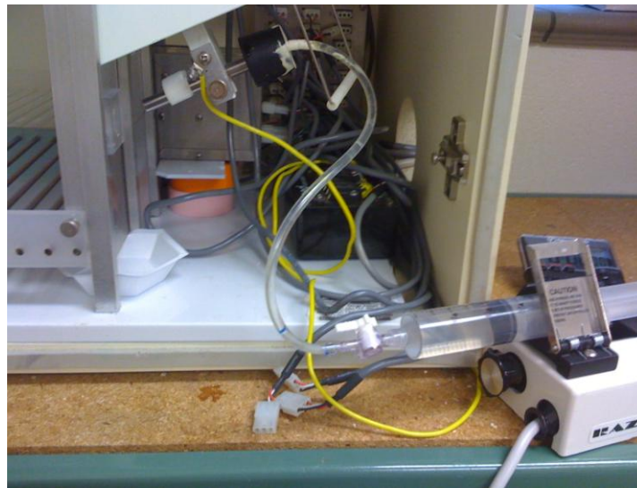
Figure 8. Placebo spout with tray underneath wall of chamber. The fluid collection tray was placed underneath the wall of the chamber to collect the drinking solution flowing out of the drinking spout and not consumed by the animal.
