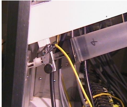
Figure 2. Placebo spout in chamber. Drinking bottle filled with 10% sucrose and placebo spout placed in chamber. The tip of the spout was inside the chamber, so that the animals could have access to the drinking solution. After the required response was met, the bottle with the drinking solution was delivered to the animals for the complete drink period. The filter paper was strategically placed so that it was close enough for the rats to smell it, but far enough for them not to reach it.
