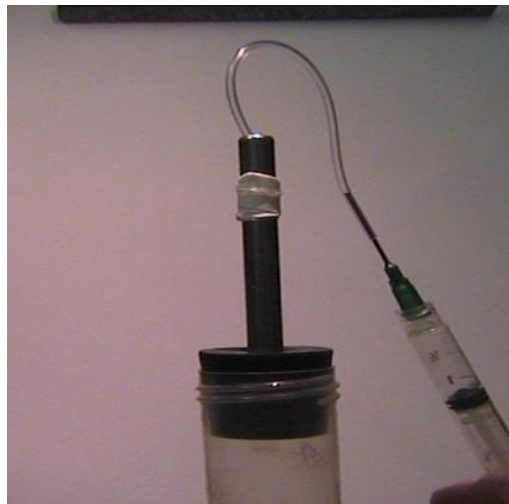
Figure 3. Placebo spout with syringe. Drinking bottle filled with 10% sucrose with rubber stopper and placebo spout. The tygon tubing was connected to the syringe to enable us to reach inside the spout completely. The syringe was used to extract the 10% sucrose solution in the spout. A similar syringe was used to add the 3.1 mls of 15% ethanol + 10% sucrose. The filter paper was saturated with 10% sucrose + 10% ethanol.
