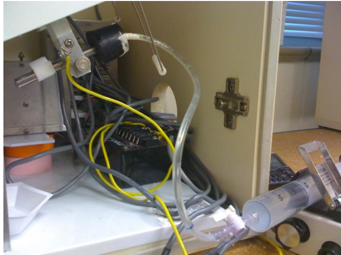
Figure 7. Placebo spout. The 30 ml syringe was filled with 25 ml of 10% sucrose and placed on a pump. A three way valve connected this syringe to another syringe containing 2.3 ml of 10% ethanol + 10% sucrose and to the tygon tubing in the drinking spout. The 10% ethanol + 10% sucrose solution was pushed into the tygon tubing, followed by air, and the 10% sucrose solution during the drinking session.
