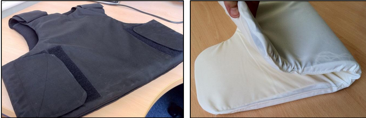
Figure 1 – Soft Body Armour Example: Stab-Resistant Duty Vest carrier (L) and aramid-based insert (R) Courtesy of Keltic Clothing [12]
