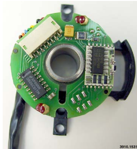
Figure 1. 200 kHz Renco encoder
