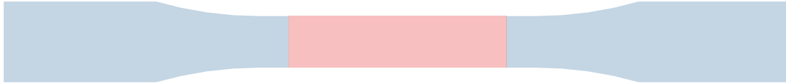
Figure 1 An illustration of dense & sparse infill regions within the tensile specimen. Sparse region shown in red, dense regions shown in blue.
