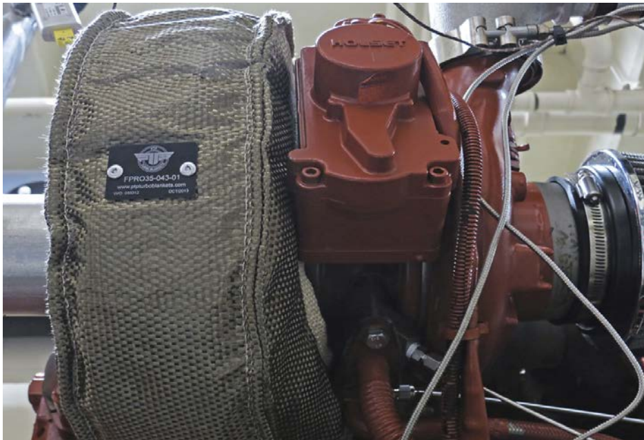
Figure 2-2 Unchanged tight fit of the PTP turbo blanket with temperature probes underneath it.
