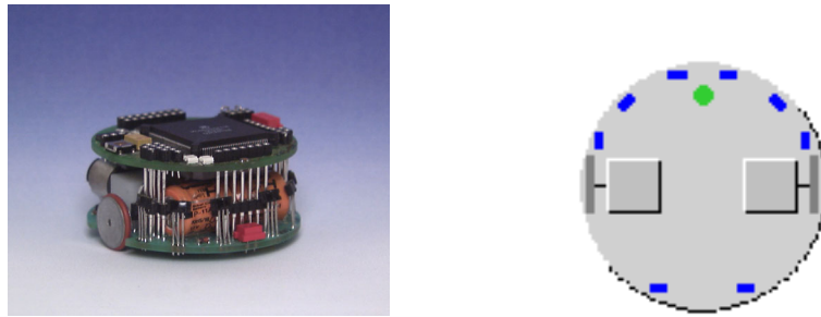
Figure 8.1: The Khepera robot, designed, manufactured and distributed by K-Team S.A., Switzerland. www.k-team.com Used by permission. The body diameter is about two inches (55 mm), and the wheels are 50 mm apart. (left) A picture of the physical robot. (right) A diagram of Khepera's floor plan showing placement of motors and wheels at left and right, and eight photosensors (blue rectangles) around the perimeter. Khepera is inexpensive and appropriate for teaching and research. Figures used with permission, copyright K-Team S.A.
