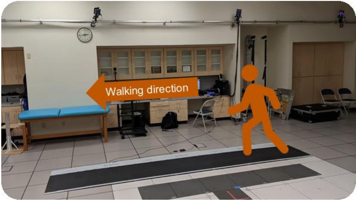
Figure 1: Photo of experimental setup within gait lab, showing Vicon Optical Motion Capture cameras mounted on overhead railings and the Strideway Gait Mat within the capture volume of the Vicon system.
