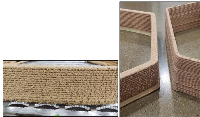
Figure 6. Initial AM samples exhibiting sharkskinning and inconsistent flow
