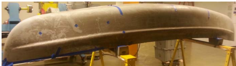
Figure 1: Canoe plug as received from MVP, in preparation for hand scanning.
