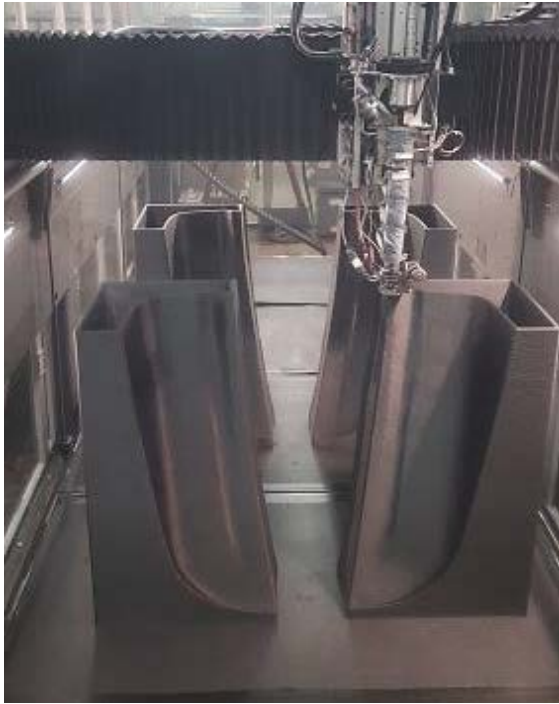
Figure 15: BAAM print underway
