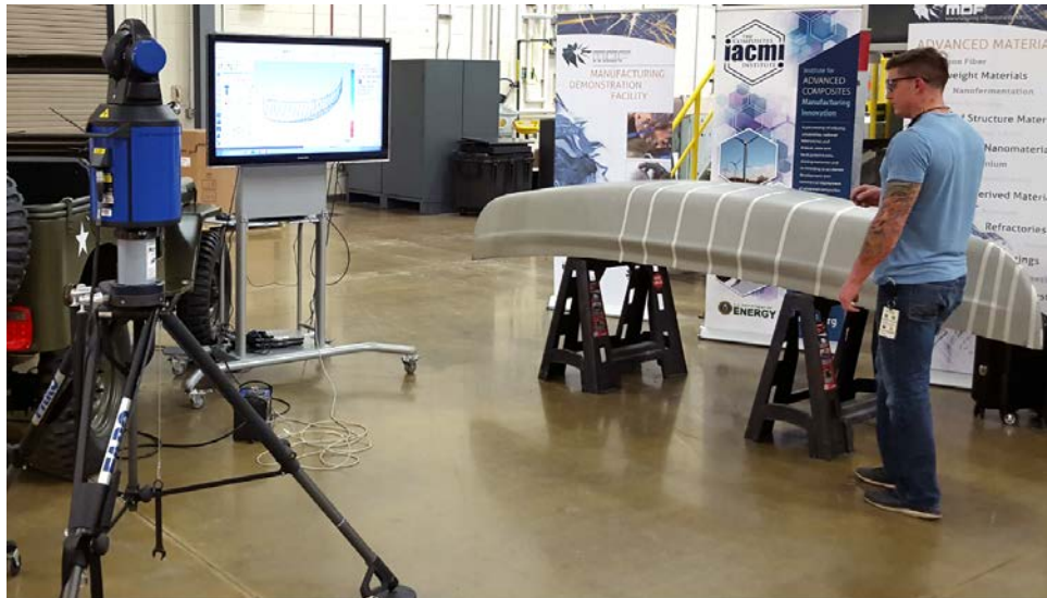
Figure 9: Laser tracker in use, tracing of the hull contour
