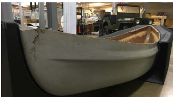
Figure 17: Bow perspective of plug fit test.
