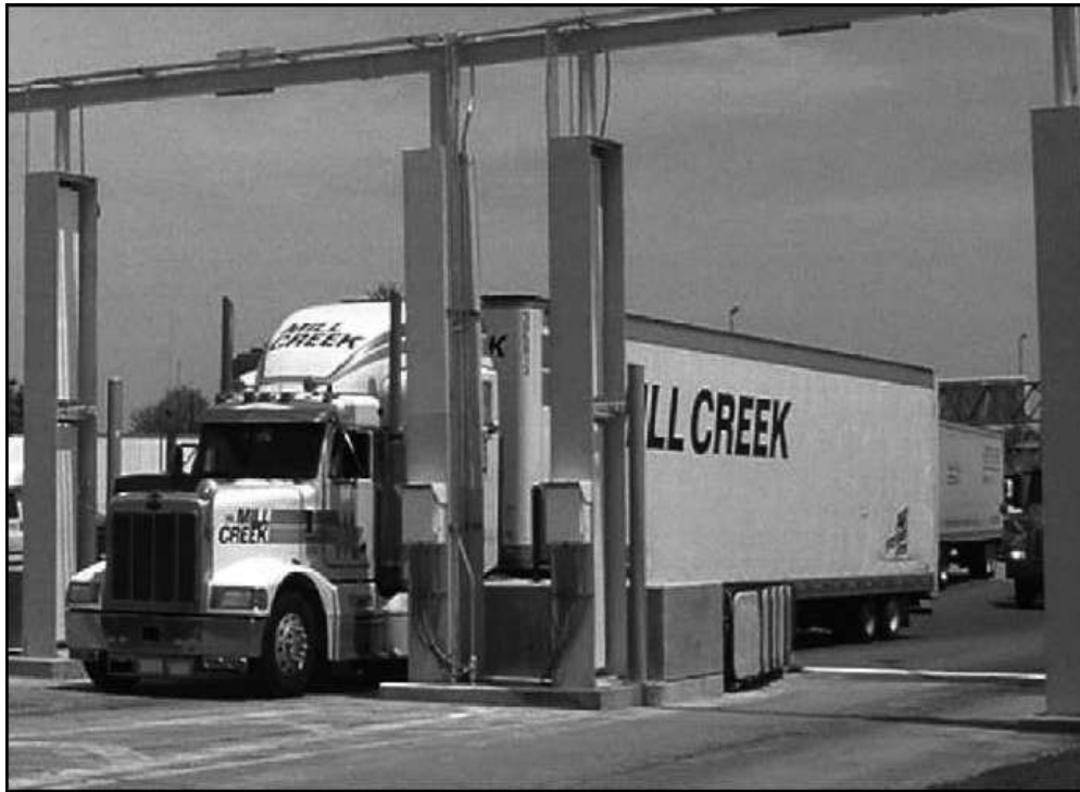
Figure 2.1: A typical RPM system for cargo screening [1]
