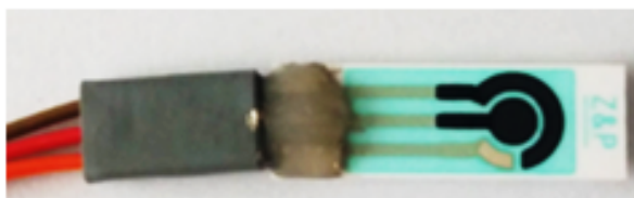
Figure 16 – Screen printed electrode, CE and WE are made of carbon and the reference electrode is Ag/AgCl.
