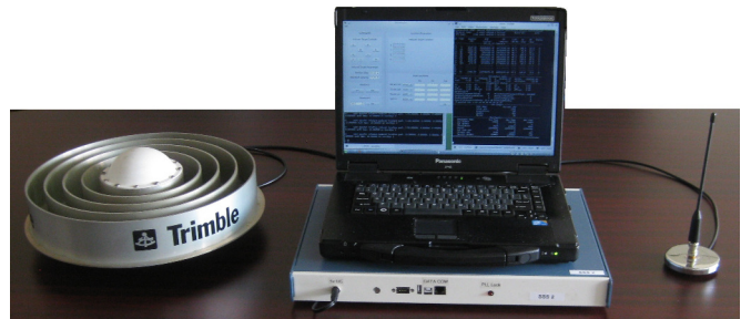
Fig. 2. The University of Texas real-time GPS spoofing device. The device as shown here is configured for over-the-air transmission but is only used as such in authorized tests [2], [3], [38]. More commonly, the spoofer’s output signals are conveyed to the target receiver by coaxial cable or digital data. The computer shown atop the spoofing device runs a client application that allows a user to monitor and control a spoofing attack over a wireless or wireline network. The client-spoofing network connection is insensitive to latencies of hundreds of milliseconds, which permits a spoofing attack to be controlled remotely over the Internet.
