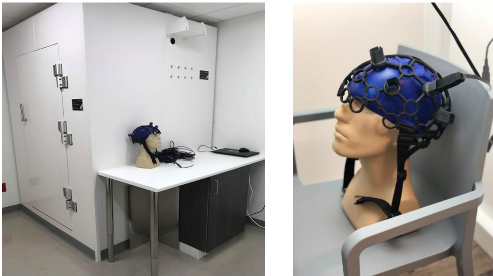
Figure 4: Examples of a magnetic shielded room for OPM-MEG (left) and an OPM-MEG helmet (right), courtesy of Dr. Davenport, UT Southwestern Medical Center
