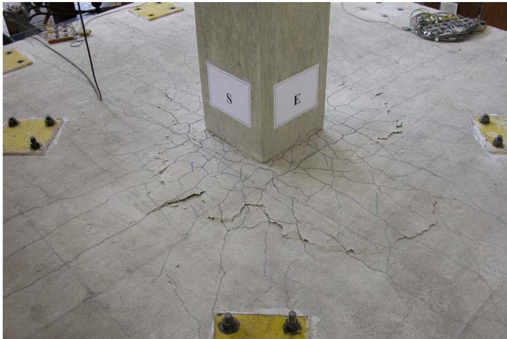
Figure B.3: Failure pattern of Specimen LG1.0.
