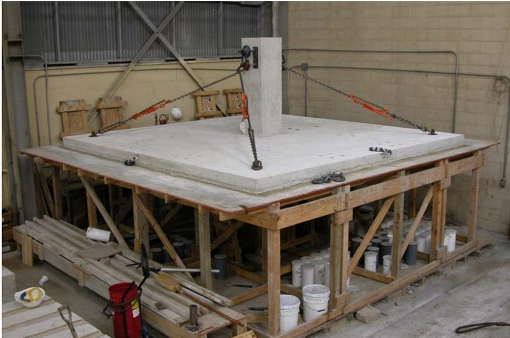
Figure 2.32: Preparation for specimen lifting.
