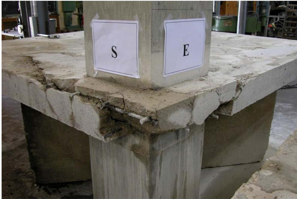
Figure B.2: Failure surface of Specimen LG0.5.
