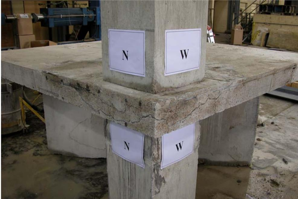
Figure B.4: Failure surface of Specimen LG1.0.
