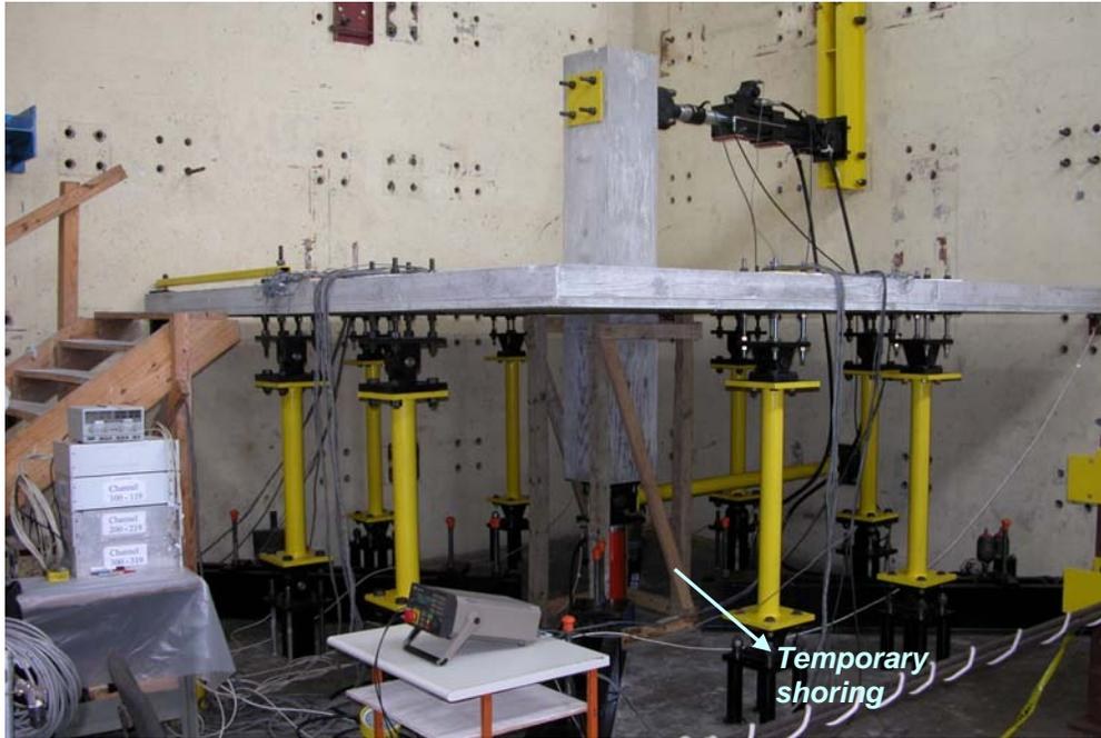
Figure 2.33: Placement of specimen in test setup.
