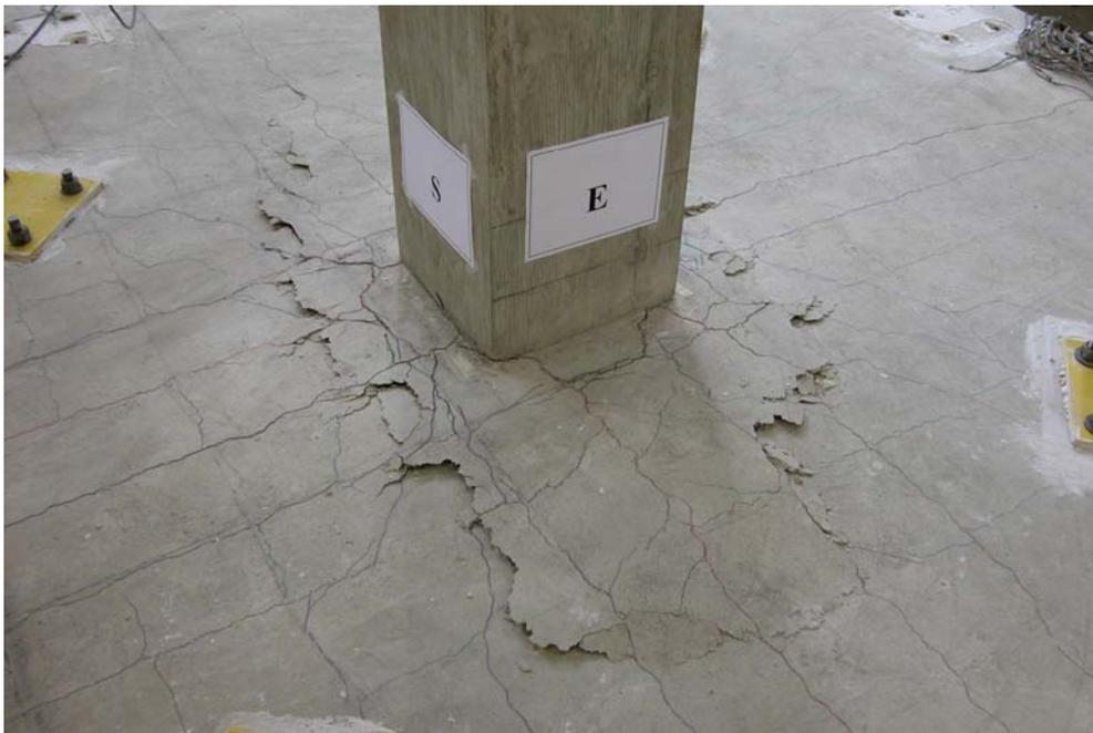
Figure B.1: Failure pattern of Specimen LG0.5.
