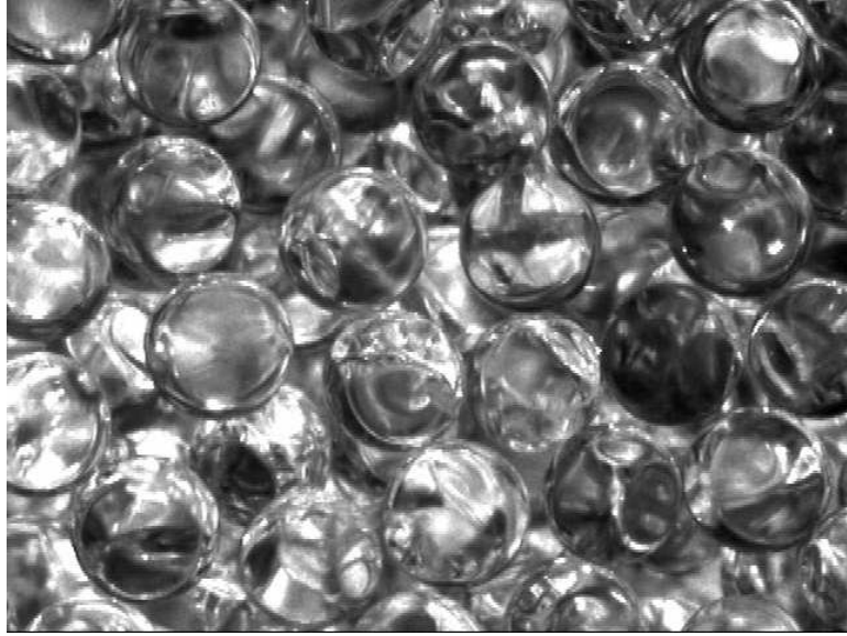
Figure 1.4: 335\ \mu\text{m} glass spheres in water
