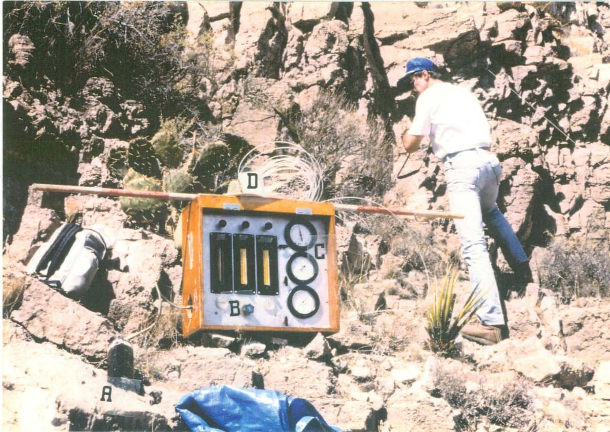
Figure 2. Mechanical Field Permeameter (MFP) used for field collection of permeability data. MFP components: A - High pressure nitrogen gas source. B - Three (3) rotameter stands to hold interchangeable flow tubes. C - Test quality pressure gage and back-up units. D - Flexible tubing with silicon probe-tip and on/off valve.
