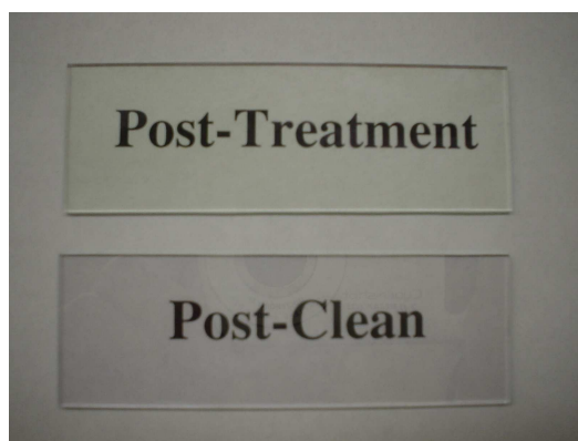
Figure 9.4: Photograph of the ITO slides before and after mechanically cleaning. The “post-treatment” sample is hazy with loosely bound material. After cleaning, the “post-clean” sample is transparent.
