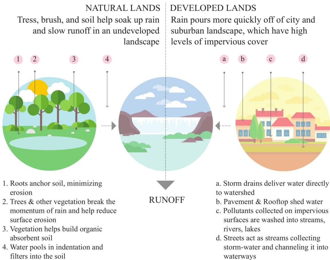
Figure 10 Impervious cover and urban drainage systems increase runoff to creeks and rivers. (Ruby, n.d.)
