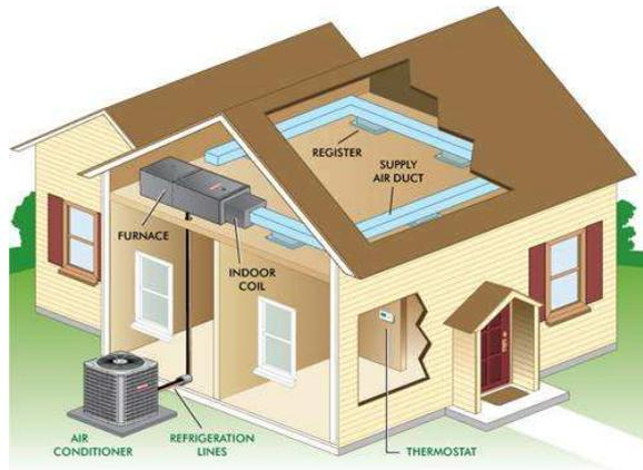
Figure 1.4: Layout of a typical residential HVAC system
