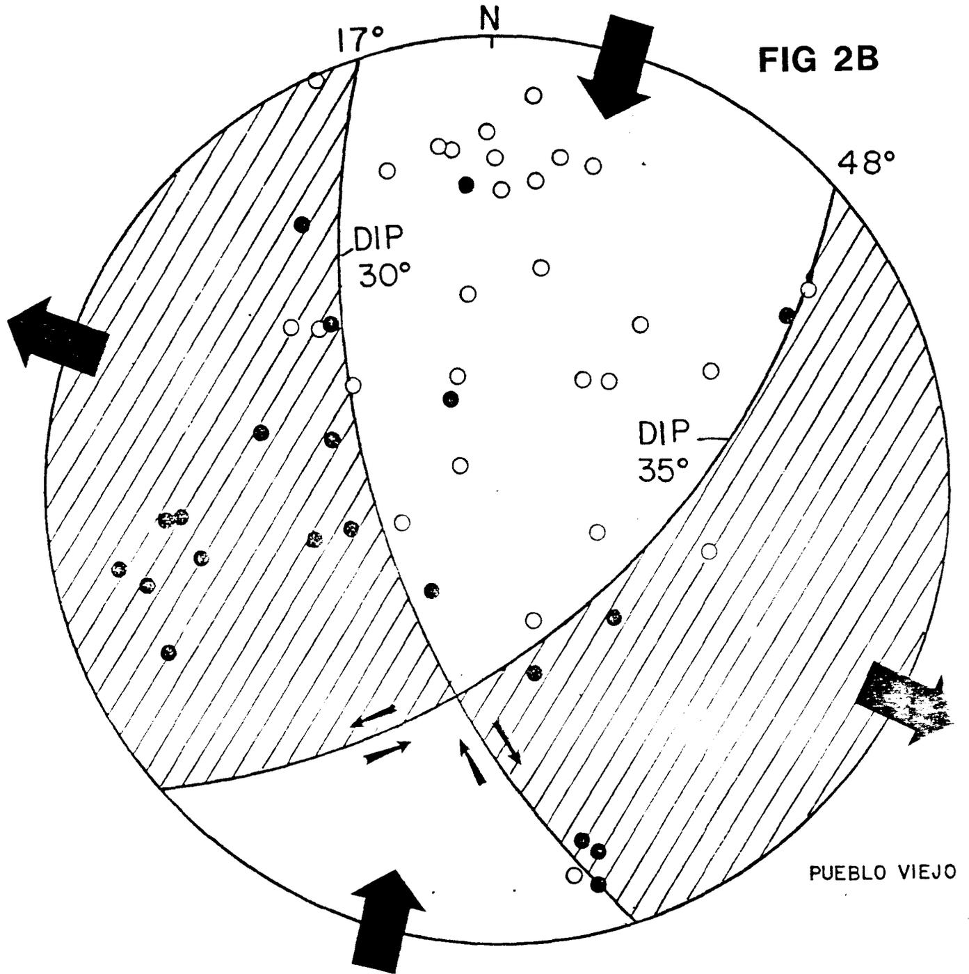
Figure 2B. Composite fault plane solution for the events in the vicinity of Pueblo Viejo Dam.
