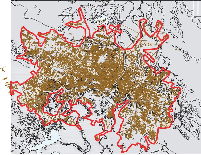
Figure 5.1: Water and wastewater service area defined by the spatial distribution of mains and sewers in Austin, Texas.
