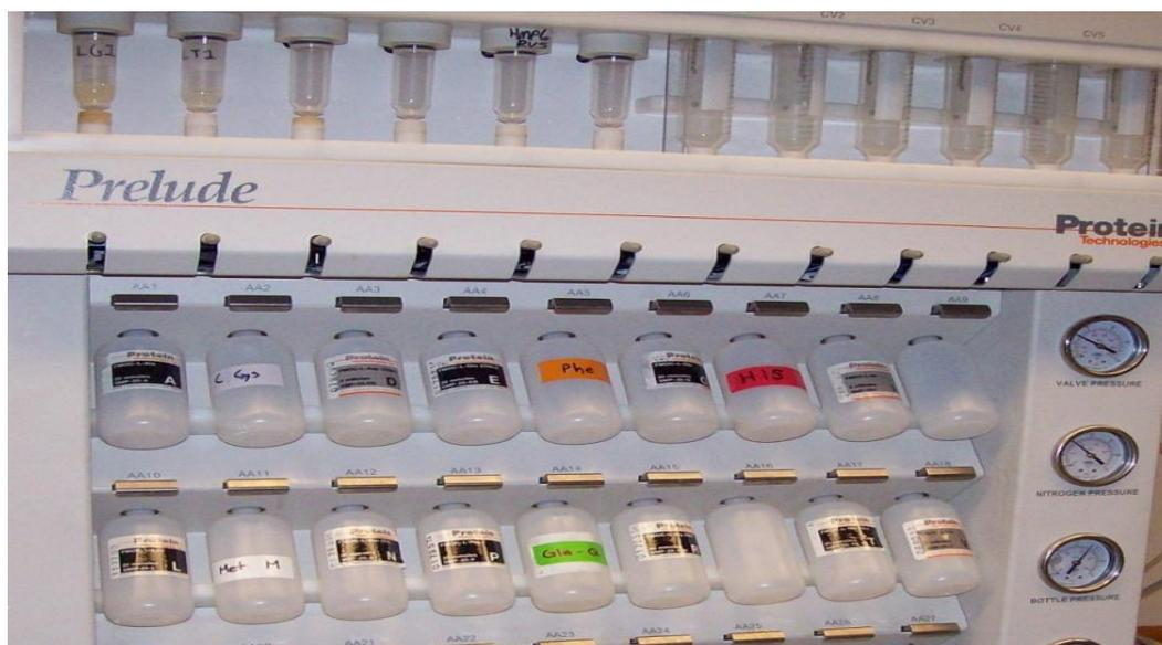
Figure: 3.3 Protein Technologies Inc. Prelude with loaded RVs.
