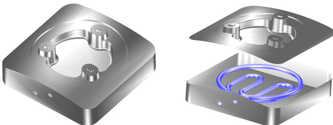
Figure 2: Left: injection molding tool insert, right: view of the internal cooling system
