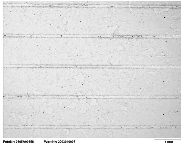
Figure 3: Cross-section of a brazed tool
