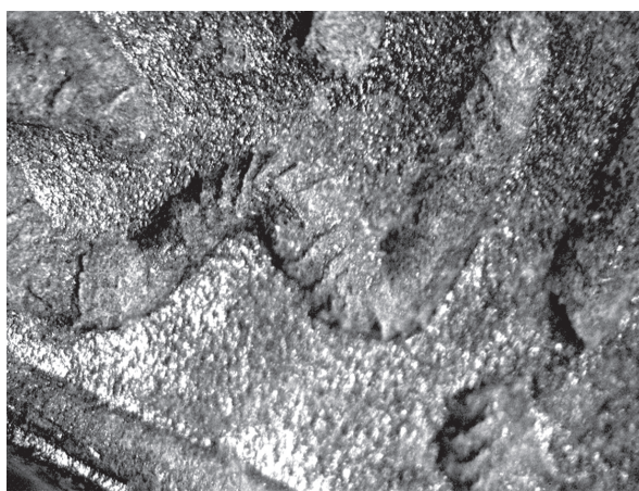
Figure 3. A photomicrograph of the lock showing engraver's tool marks.
