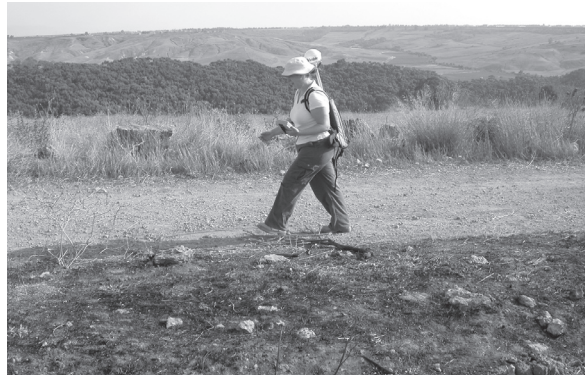
Figure 12. Plot boundaries are recorded with the most rugged and easiest-to-use of the survey GPS receivers.
