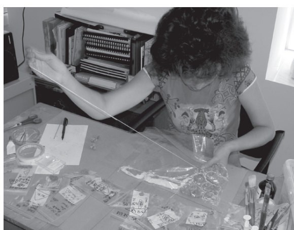
Figure 4. Inga Shvedova sews metal objects into plastic sheeting in preparation for X-ray analysis.
