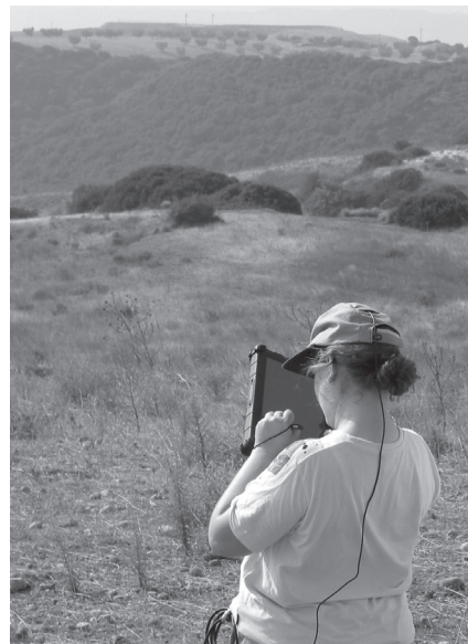
Figure 14. The smallest (pocket) receiver attaches to the Xplore tablet computer, and together they make a convenient platform for the recording of both the site-center location and the site/plot notes.
