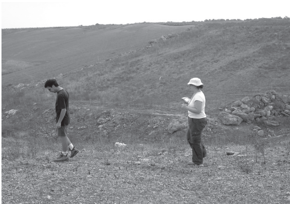
Figure 13. Site-boundary recording is best performed with the hand-held receiver, operated by a field-walker who follows a path created by one of the survey leaders.
