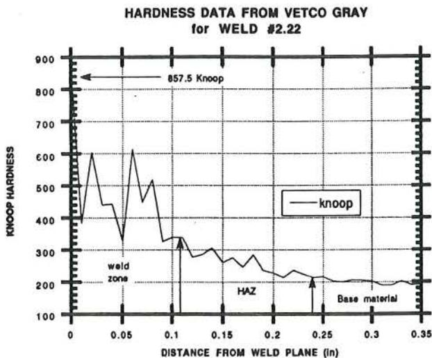
Fig. 6 Microhardness traverse of 3-in. Schedule 160 C1035 pipe weld (HPW)
