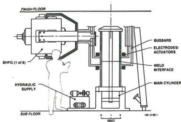
Fig. 8 Proposed 0.56 m pipe welding system powered by the BHPG power supply
