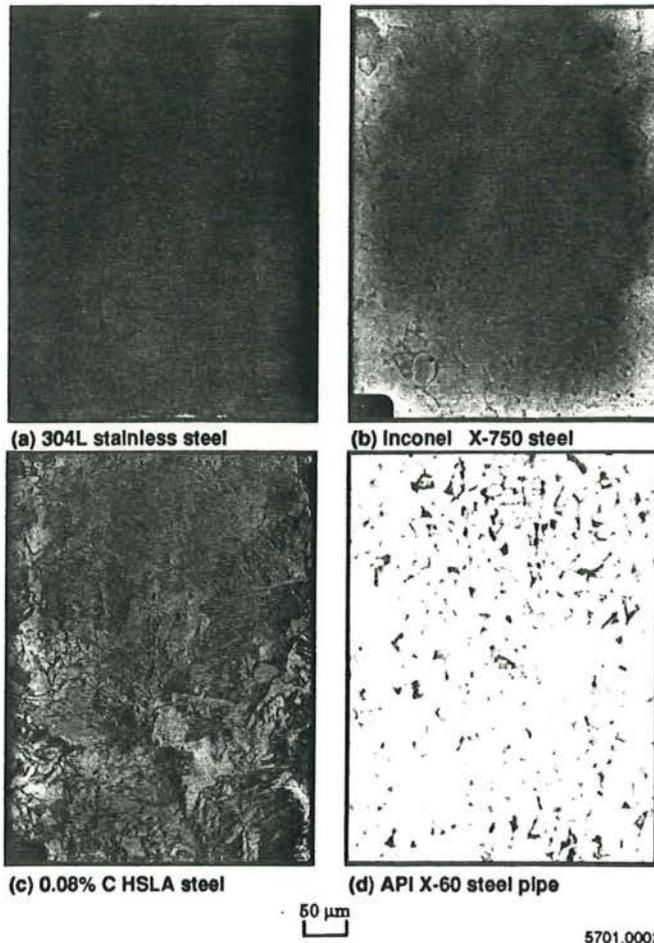
Fig. 2 As-welded microstructure of various alloys joined by HPW. Weld line centered, vertical. Etchant varies.
