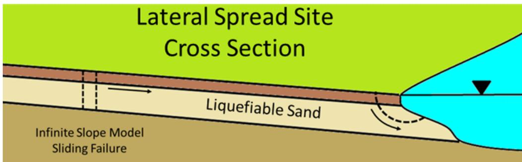
Figure 4.8: Cross sectional view of a lateral spread site with an example of where an infinite slope model would be appropriate.
