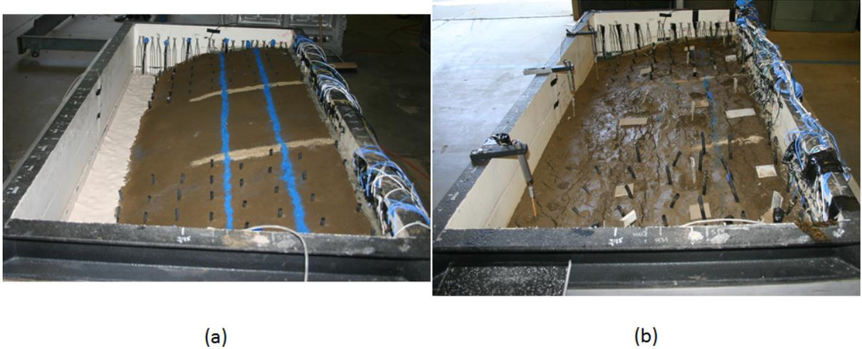
Figure 3.28: The RLH01 centrifuge model (a) before shaking and (b) after shaking.
