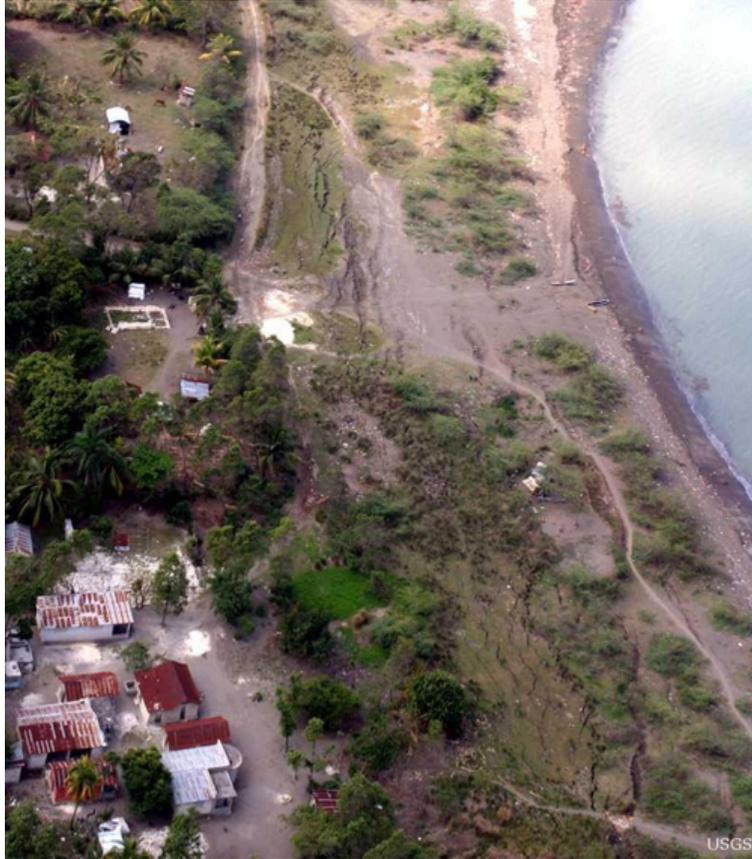
Figure 1.2: Aerial photograph of a lateral spread site in Port Au Prince, Haiti, taken by the U.S. Geological Survey after the 2010 earthquake (USGS, 2013).
