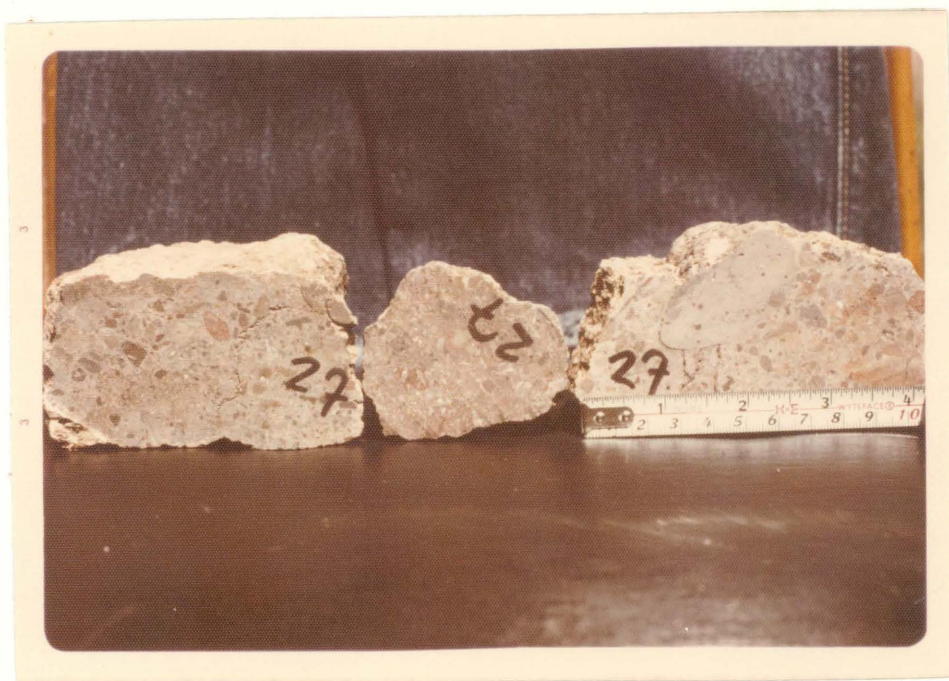
Fig. 13. Hand specimens of agglomerate exposed within diabase plug north-northwest of Hill 3412 (EC). The rock is mostly basaltic volcanic rock fragments cemented by analcite. Some larger rock fragments are well-rounded.
