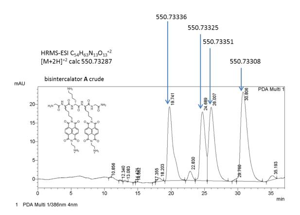
Figure 2.8: Crude solution of bisintercalator **A** run on Shimadzu LCsolution HPLC after synthesis using old SPPS protocol. Indicated peaks were isolated and observed HRMS-ESI values reported above respective peaks.
