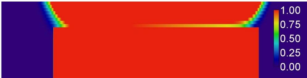
Figure 2.3 Melt fraction when applying a constant laser power to powder with non-constant temperature
