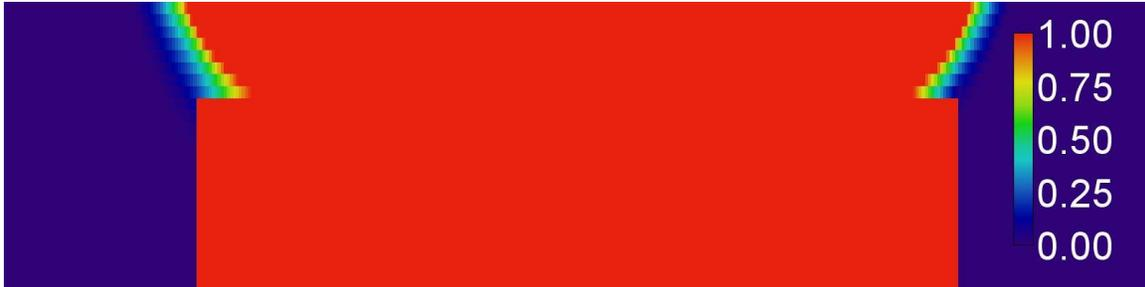
Figure 2.4 Melt fraction when applying a variable laser power to powder with non-constant temperature
