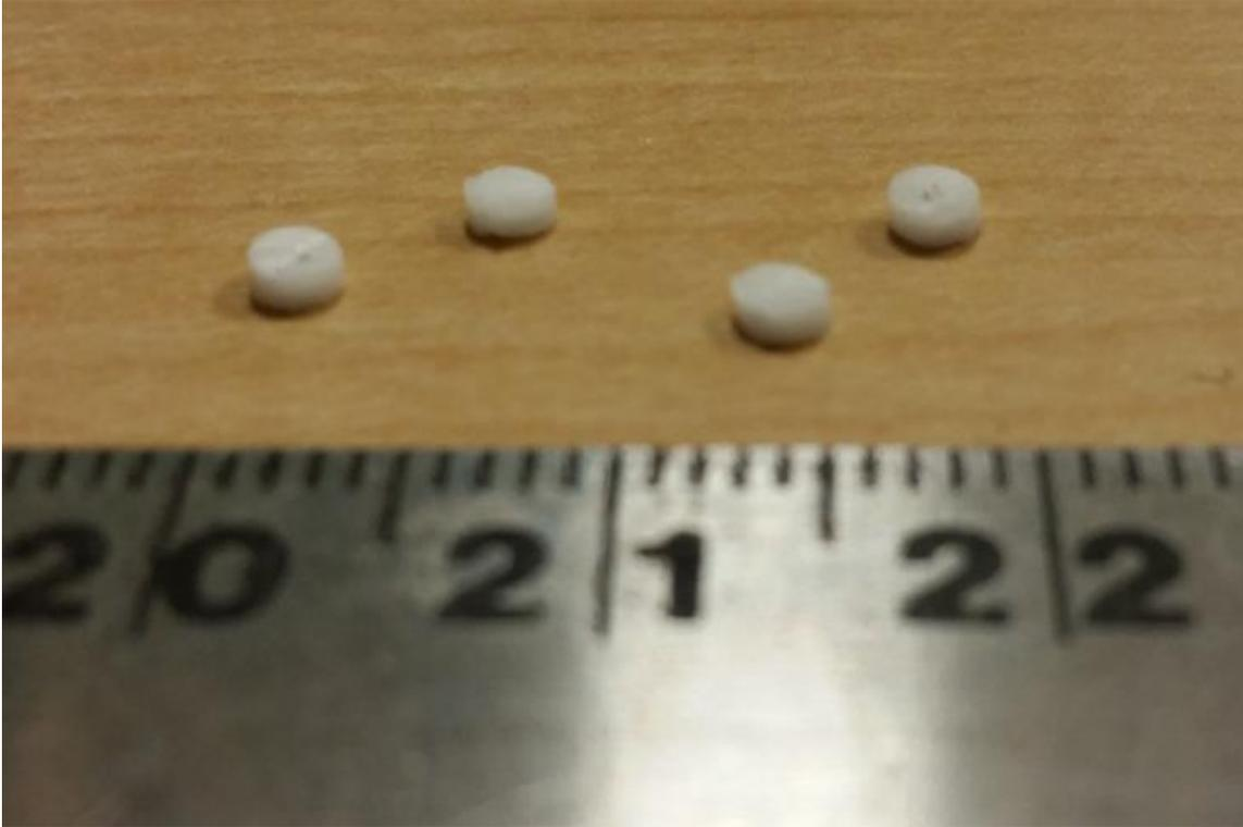
Figure 4.8 Nylon 12 samples prepped for DSC
