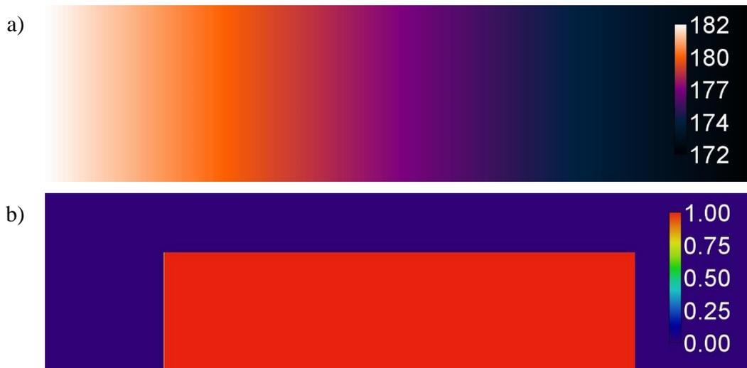
Figure 2.2 Initial conditions of thermal simulation showing a side view of (a) starting temperature and (b) starting melt fraction
