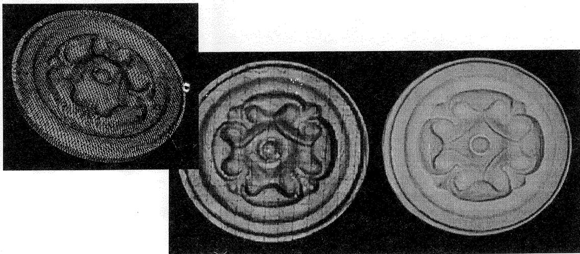
Figure 1. Computer file (inset) obtained from Photogrammetry techniques. LOM master pattern (left), original plaster item (right).
