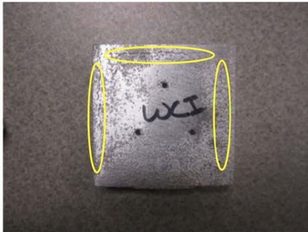
(a) White cast iron tile encapsulated in Al-Cu alloy exhibiting hot tearing
