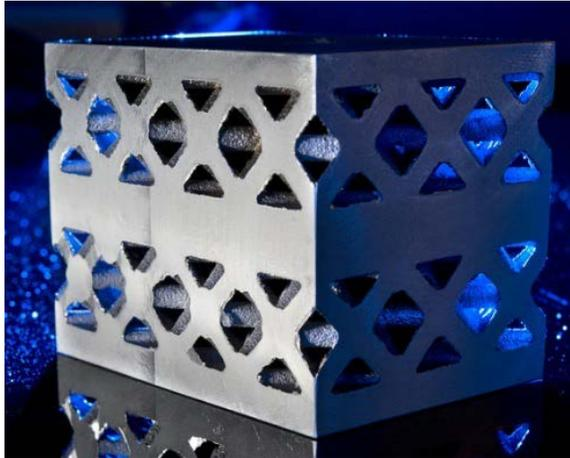
**Figure 3.** Cast lattice structure resulting from a 3D printed sand mold.
