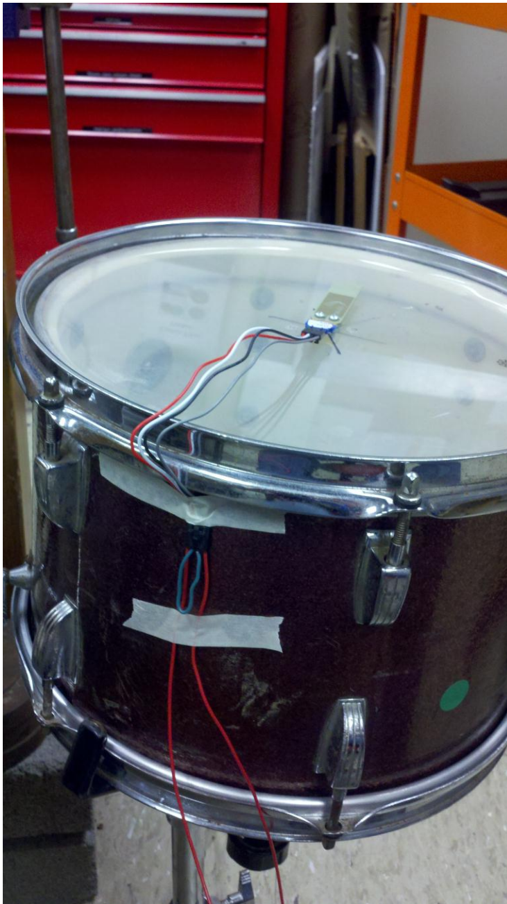
Figure 10: The harvester, attached to the bottom of the small drum (the drum is currently upside down) with a 4 pin connector ending in one output and one input wire.
