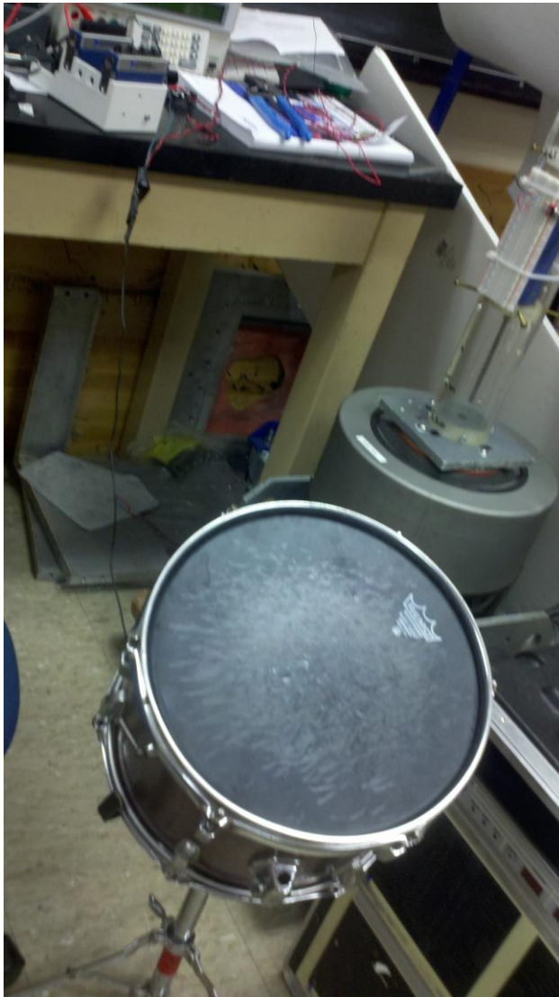
Figure 1: The Ludwig, or “small drum” shown with the accelerometer underneath connected to the NI cDAQ in the upper left corner.
