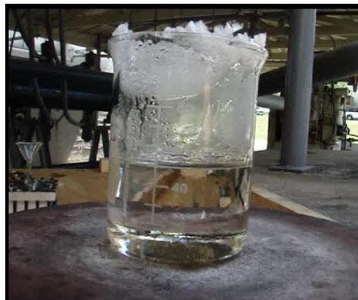
**Figure 3.3 Naphthalene crystals melting on a hot plate**
