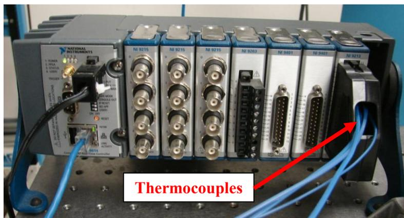
**Figure 3.15 Compact RIO System with thermocouples**
