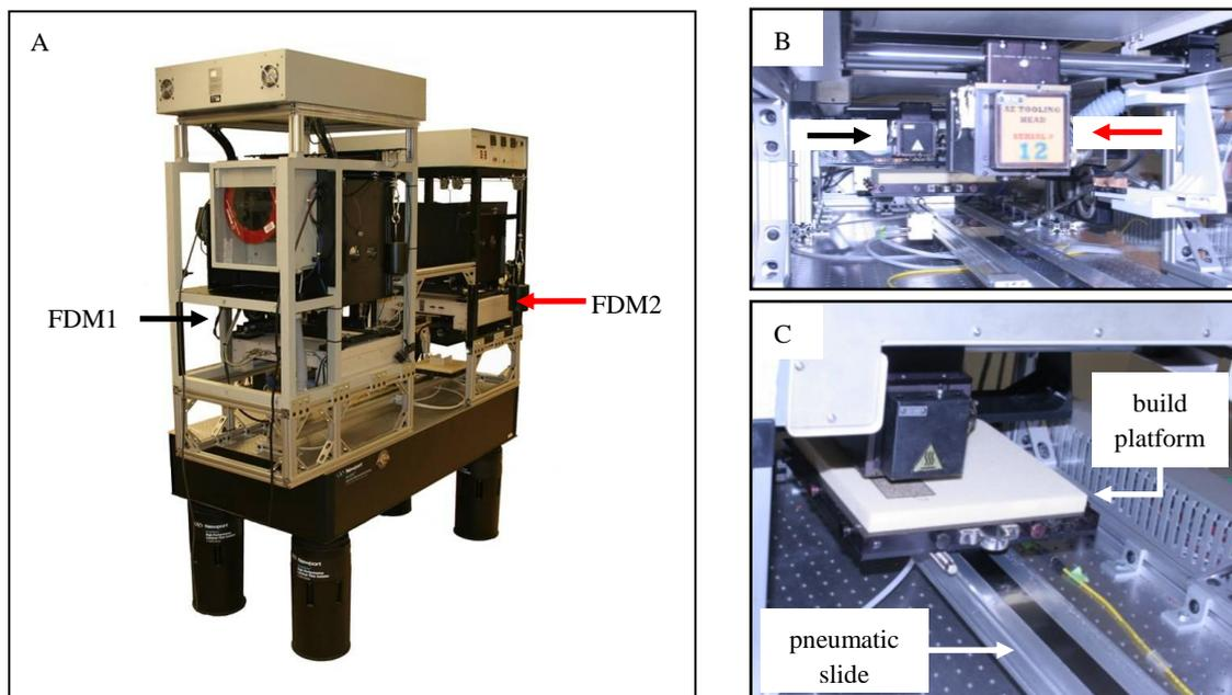
Figure 3: Multi-material, multi-technology FDM system. A) overview of entire system. B) inside view of build envelope (note that FDM1 and FDM2 are highlighted by a black and red arrow, respectively). C) close-up view of FDM1 building on the platform that is attached to a pneumatic slide.
