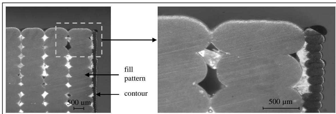
**Figure 6:** Cross section of square prism obtained with optical microscopy (overview on left and close-up on right). Note the fill pattern is made with a large layer thickness and road width while the contour is made with thinner layer thickness and road width.
