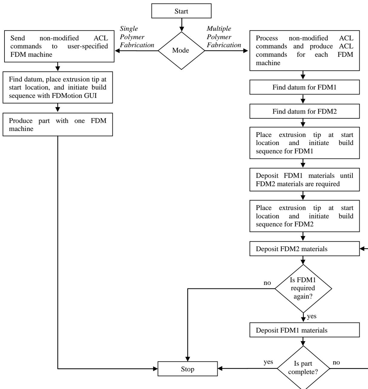
Figure 5: Block diagram for sequence of actions performed by FDMotion.
