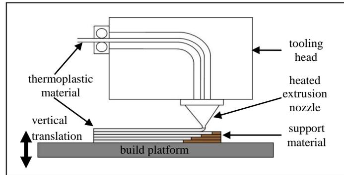
**Figure 1: Schematic of FDM process for legacy systems.**
