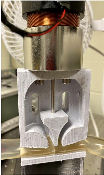
Figure 8.1: Prototype Cardiac Event Generator (CEG) for high frequency arrhythmia generation and suction event implementation.
