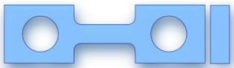
Figure 2: Schematic representation of designed miniature pin-loaded tensile test specimen with 3.3 mm gage length and 17.7 mm of overall length
