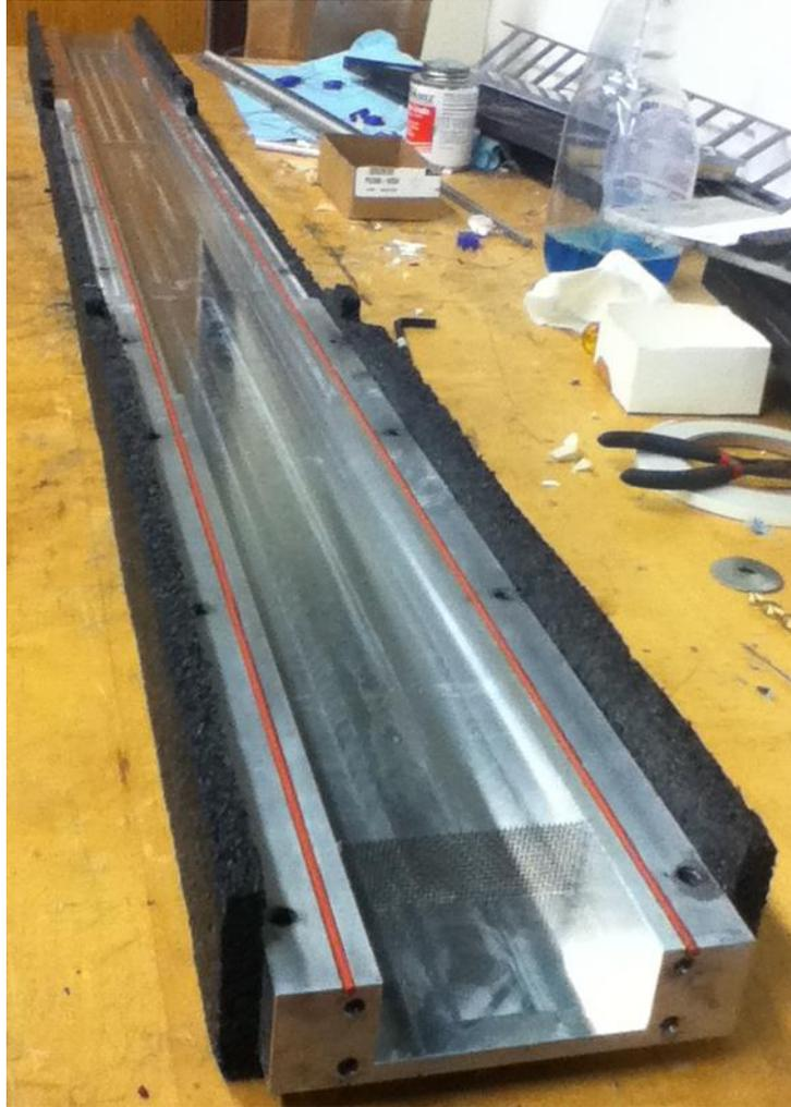
**A.1: Picture of disassembled channel with silicone cord stock o-ring.**
