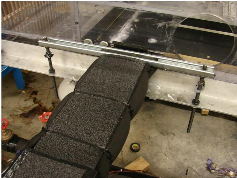
**Figure 2.18: Channel leveling system.**
