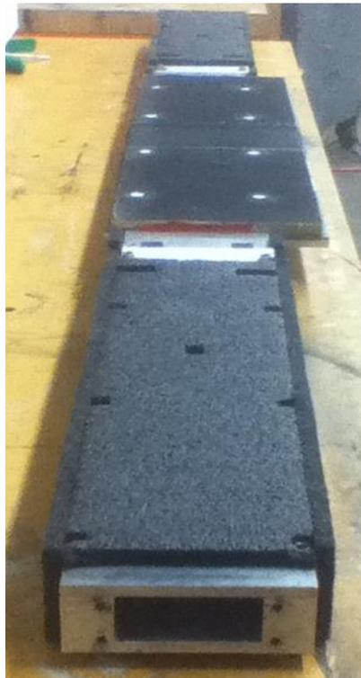
**Figure 2.17: Assembled channel and test coupon. A layer of black insulation was adhered to the aluminum to constitute a first layer of insulation.**
