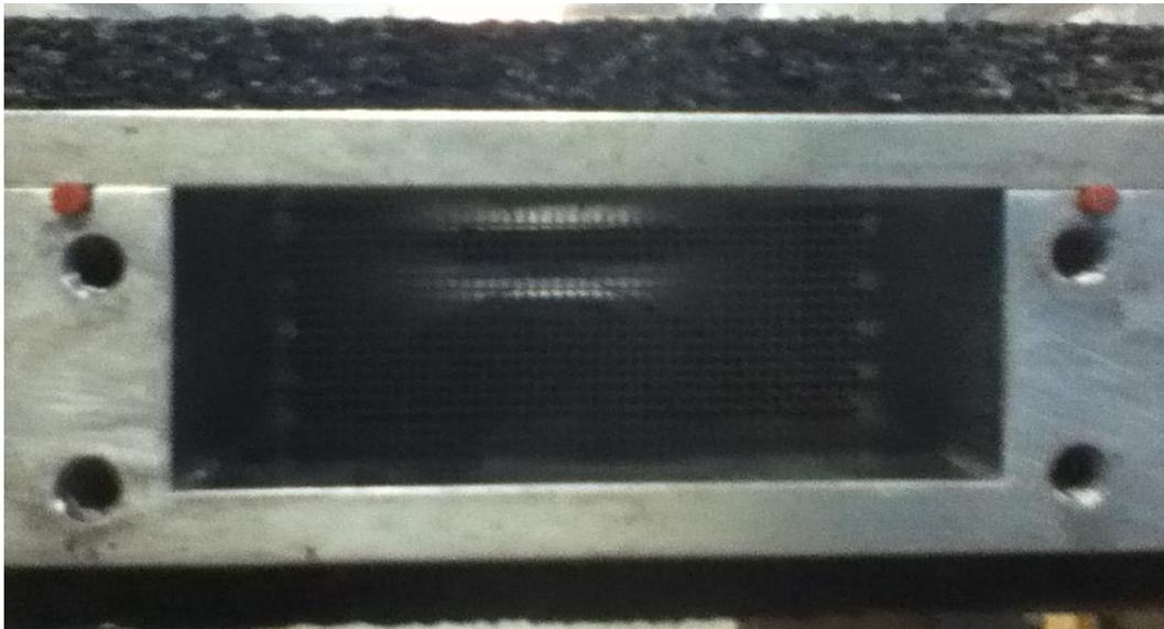
**Appendix A.3.: Internal view of channel including the internal flow straightening screen**
