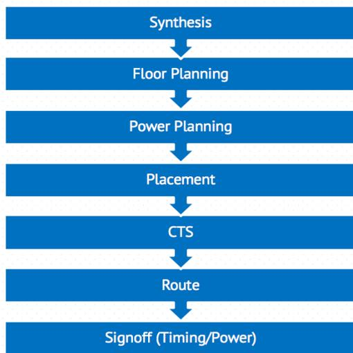
Figure 7: ASIC EDA Design Flow.
