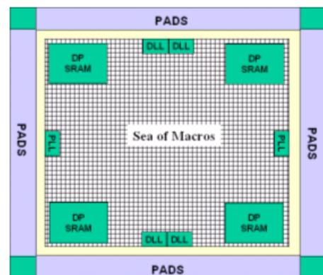
Figure 4: Structured ASIC architecture [10].
