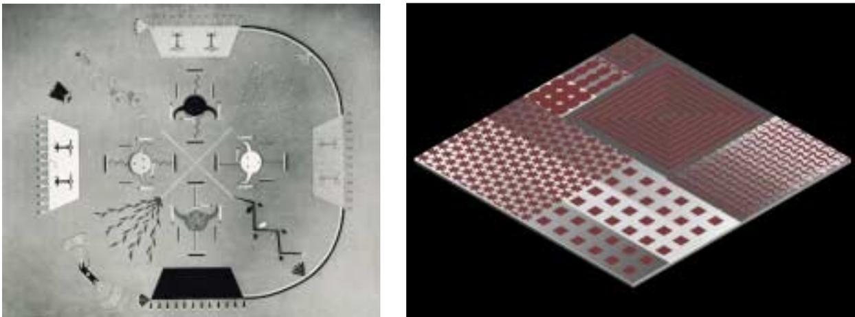
Figure 1. (a) Navajo sand painting, The Arizona State Museum, University of Arizona and (b) Conceptual design of a multiple material, patterned, powder layer for building multifunctional components by SLS.
