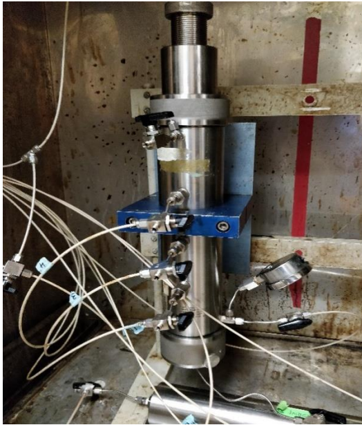
Figure 3.13. Coreholder used for coreflood experiments at various reservoir temperatures
