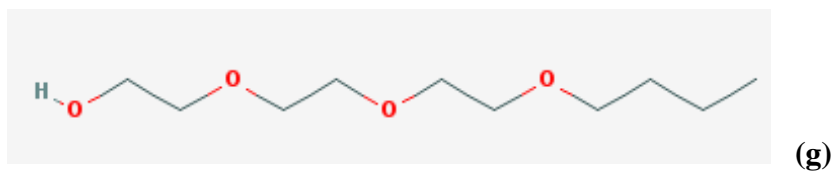
Figure 3.2. Surfactant structures for (a) TDA-xPO-yEO-SO 4 (b) Oleyl-xPO-yEO-SO 4 (c) Guerbet-xPO-yPO-SO 4 (d)Tergitol NP-10 (e) Lauryl betaine (f) Cocoamidopropyl hydroxysultaine (g) TEGBE
