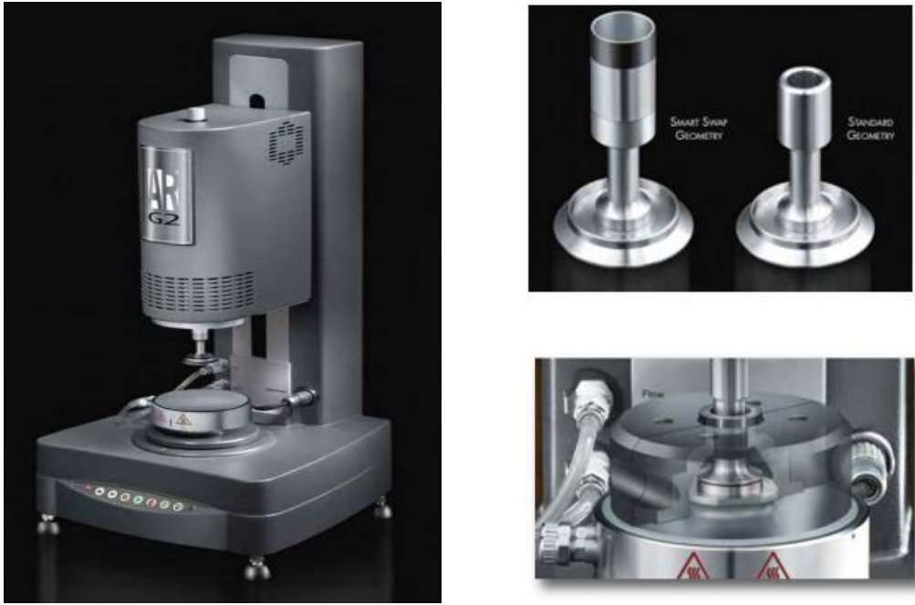
Figure 3.11. TA Instruments AR-G2 rheometer (left) and standard geometry and thermal insulation cover (right)
