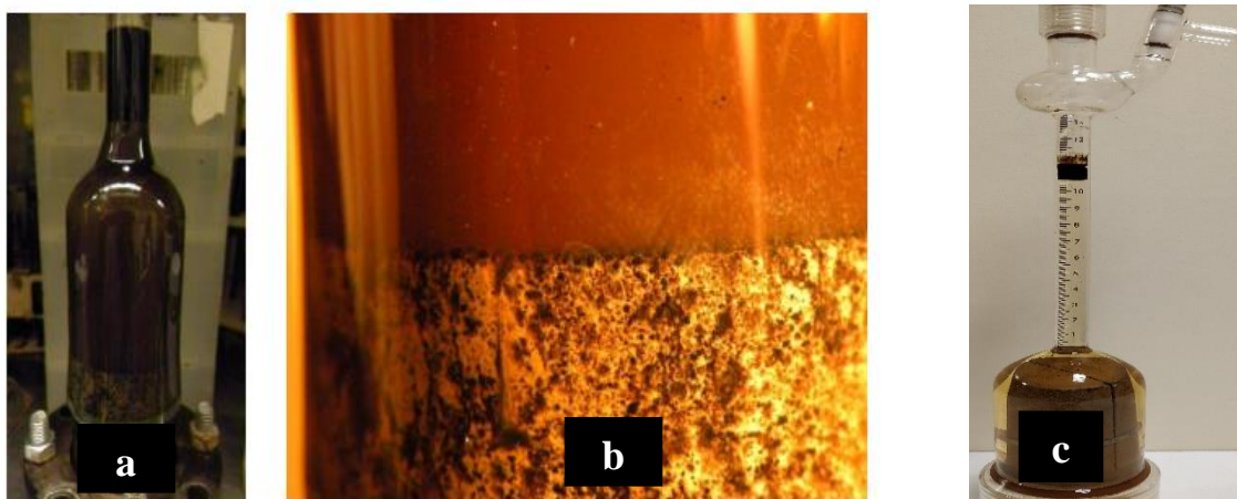
Figure 4.5. (a) Oil recovery by surfactant formulation S1 in the imbibition cell after 10 days (b) the close-up picture of the core (c) oil recovery by formulation S2 in the imbibition cell after 8 days
