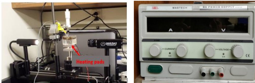
Figure 3.4. A snapshot of the Rame Hart Goniometer (left) and voltmeter used to control the temperature of the heating pads (right)
