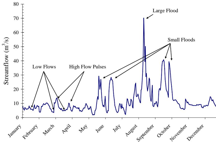
**Figure 4-17** 75% Daily streamflow hydrograph representation
