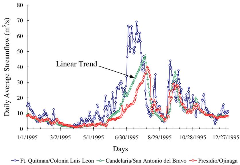
**Figure 4-4** Hydrographs of daily flow for the three gages on the Forgotten River for the year 1995
