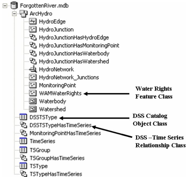
**Figure 3-10** Contents of the final Forgotten River Arc Hydro geodatabase
