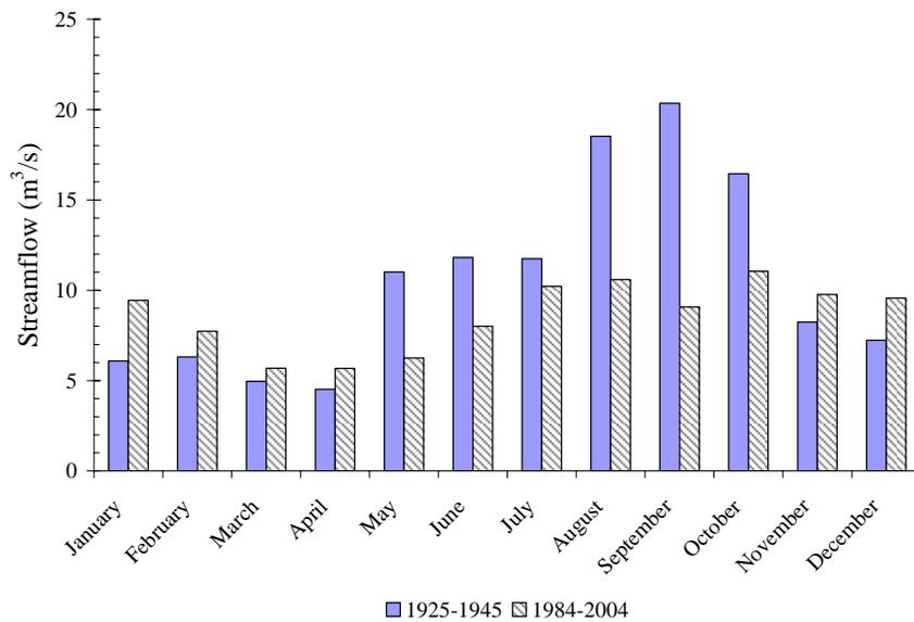
**Figure 4-11** Two period comparison of the average monthly streamflows for the Presidio/Ojinaga gage
