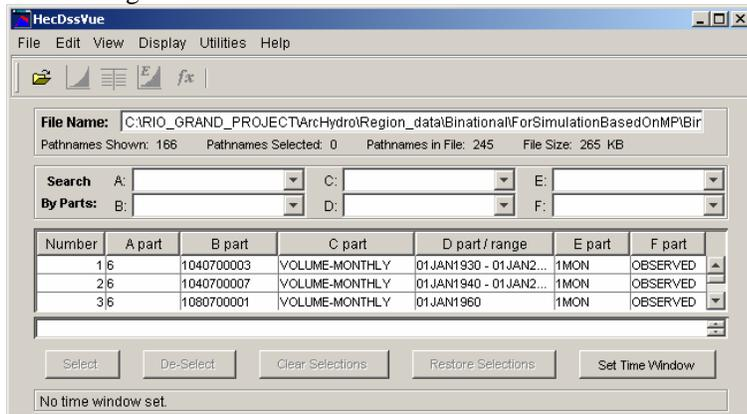
3. Transfer HEC-DSS Time Series to the GDB without Filter. This option transfers ALL temporal information from the HEC-DSS files to the GDB.
