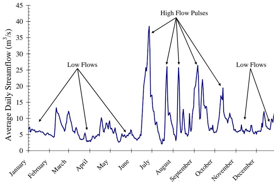
**Figure 4-16** 50% Daily streamflow hydrograph representation
