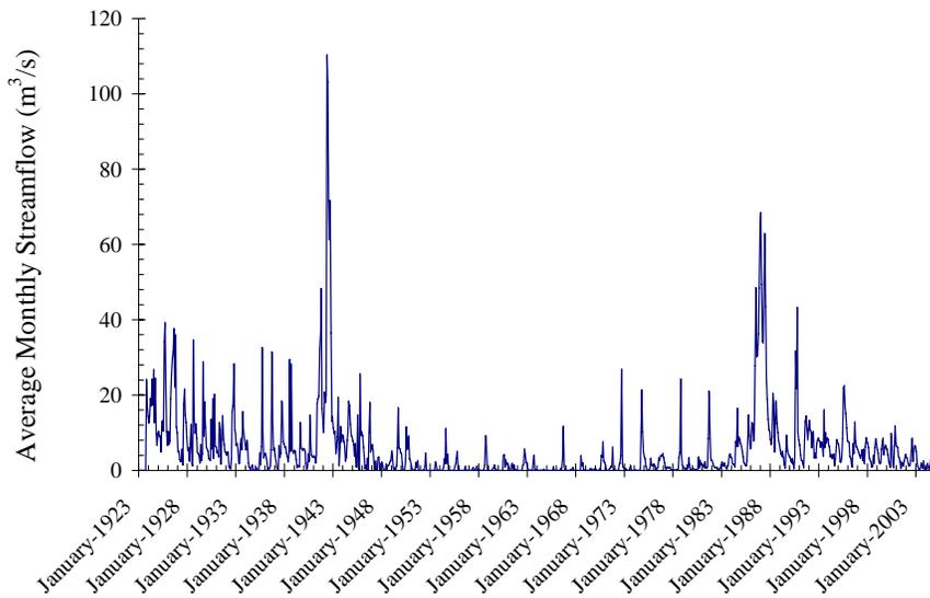
**Figure 4-3** Average monthly streamflow at Presidio/Ojinaga calculated from average daily streamflow (IBWC, 2004)
