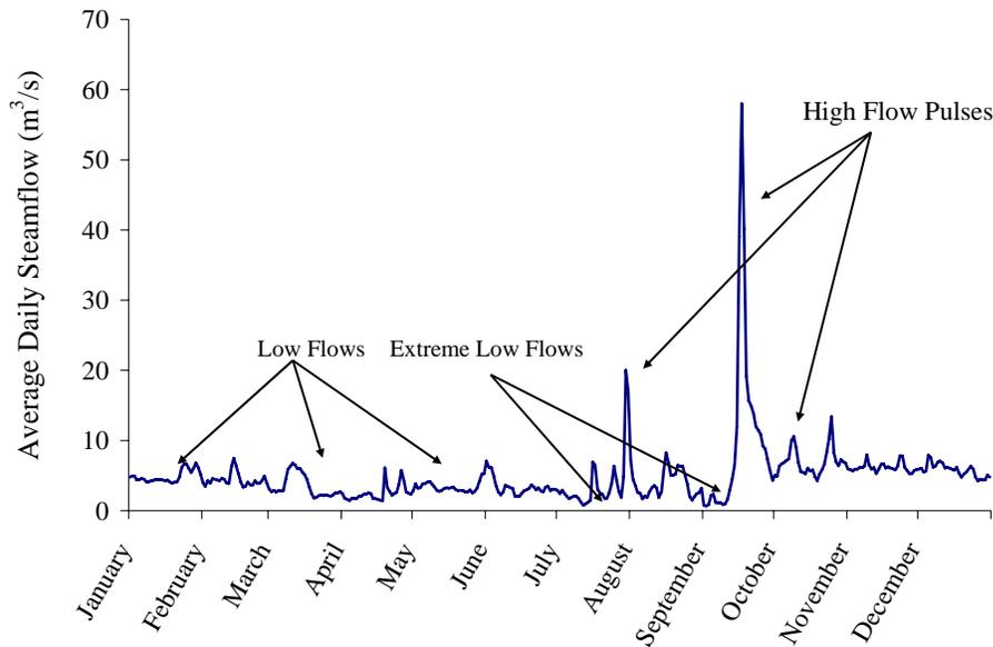
**Figure 4-15** 25% Daily streamflow hydrograph representation
