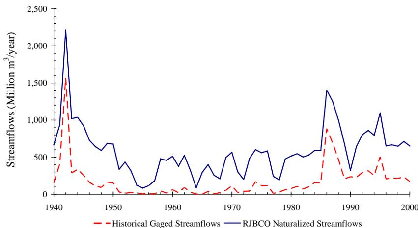
**Figure 3-13** Comparison of WAM naturalized flows with gages streamflows at the Fort Quitman/Colonia Luis Leon gage (adapted from RJBCO, 2004)
