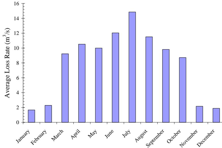
**Figure 4-19** Calculated average losses time series for the period 1984-2000
