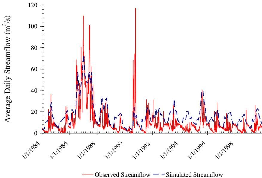
**Figure 4-18** HEC-ResSim simulated daily streamflows vs. observed daily historical streamflow values at the Presidio/Ojinaga gage
