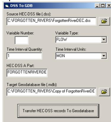
Choose the HEC-DSS file from where you want to transfer the information. Select the number variable appearing in the A Part of the HEC-DSS file (Number 6 in this example). Select the Variable Type that should be the same appearing in the C Part of the HEC-DSS file (VOLUME-MONTHLY). Select the time interval units, and type the HEC-DSS A Part (6 for this example, and it must be the same value as appears in the
