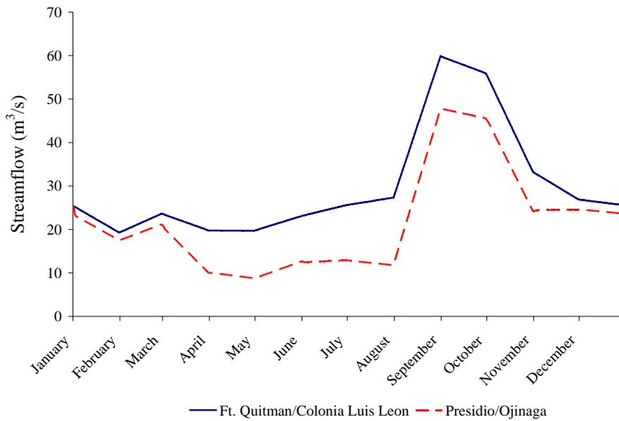
**Figure 4-23** HEC-ResSim results for the 75% recommended hydrograph
