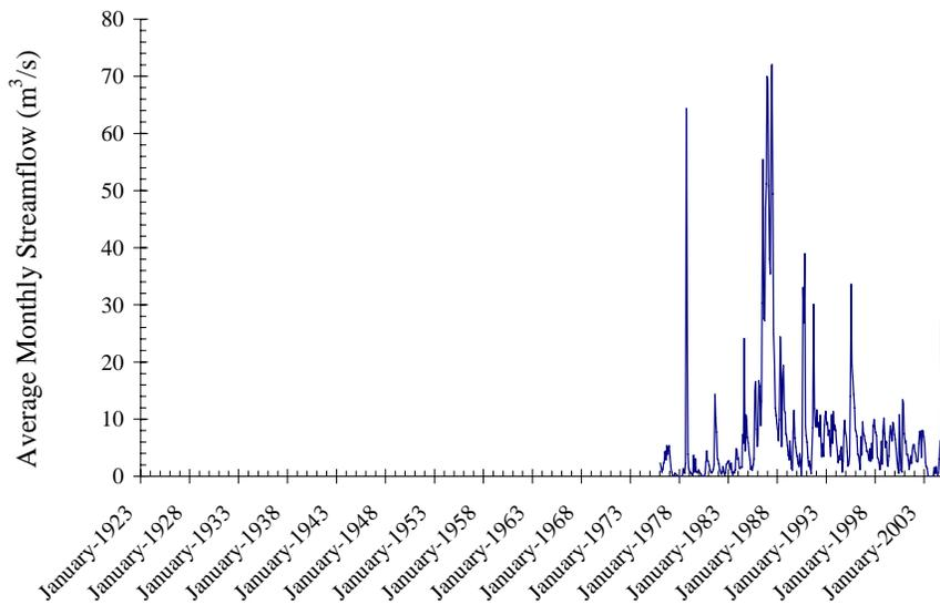
**Figure 4-2** Average monthly streamflow at Candelaria / Colonia Luis Leon calculated from average daily streamflow (IBWC, 2004)
