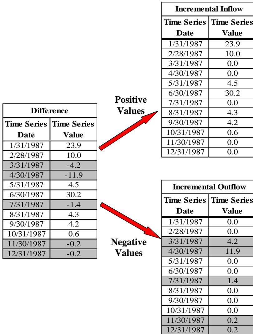
**Figure 3-12** The difference time series is split into two new time series, one for the positive values and one for the negative values, to represent incremental inflow (positive) and incremental outflow (negative).
