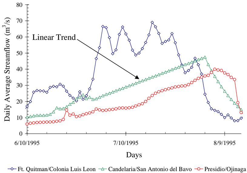
**Figure 4-5** Hydrographs of daily flow for the three gages on the Forgotten River for the year 1995
