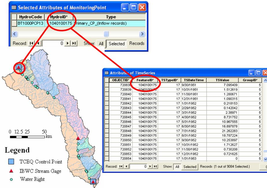
Figure 3-5 Arc Hydro relationship establishes a connection between a Control Point in the Monitoring Point feature class and the time series object class
