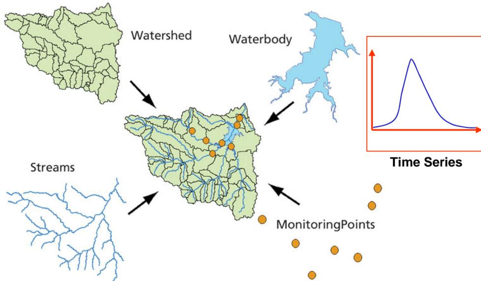
**Figure 2-3** Arc Hydro data model framework with time series (Maidment 2002)
