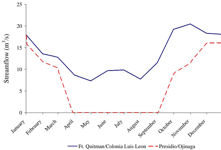
**Figure 4-21** HEC-ResSim results for the 25% recommended hydrograph
