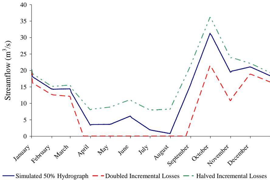
**Figure 4-24** Resulting hydrographs at Presidio/Ojinaga from changing the incremental losses
