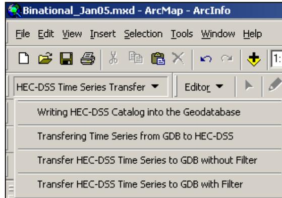
1. Writing HEC-DSS Catalog into the geodatabase: This option allows populating automatically the DSSTSType table, which was created previously by the ArcHydro schema. This function takes the temporal information from the Time Series and the TSType tables included in the ArcHydro geodatabase. The TSType table must have the next structure in order to be able to transfer the temporal information.
