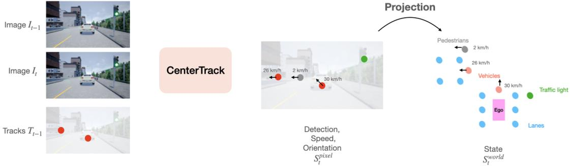
Figure 4.2: **Perception module** – Our perception module follows CenterTrack [46]. It takes current and previous observations as well as previous track as input and predicts current object location, orientation and speed (displacement) in pixel coordinates. Then, we project from pixel to world coordinates using known camera intrinsics and extrinsics.
