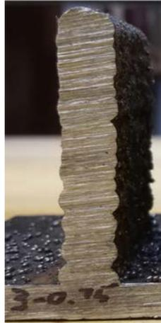
Figure 10. 410 stainless steel, two-bead thick wall without any voids
