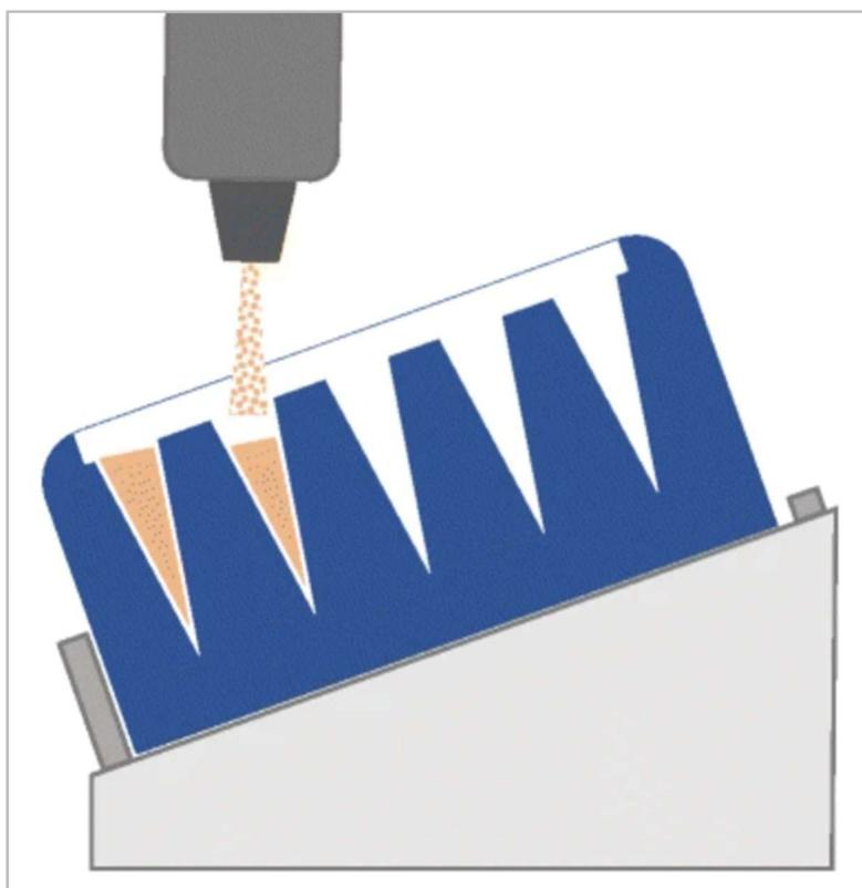
Figure 1.5 More recently utilized dispensing methods for micromold filling such as atomized spraying or inkjet printing eliminate the need for a separate centrifugation or vacuuming step to remove trapped air from the molds, thereby improving not only the accuracy and precision of the microneedle manufacturing process, but also the translation to continuous manufacturing, which is readily scalable. (Reproduced with permission from Springer Nature)
