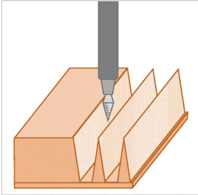
Figure 1.4 Micromilling to produce master molds uses ultrahigh speed, high precision, rotating single-crystal diamond cutting tools to machine microneedle designs out of a hard substrate such as PMMA (or PLGA, metal, or ceramic) within minutes to hours. (Reproduced with permission from Springer Nature)
