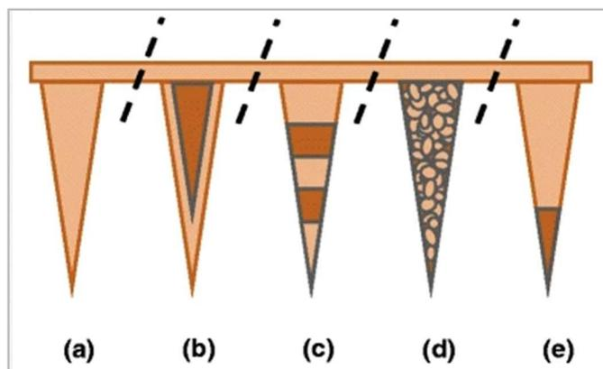
Figure 1.2 Dissolving microneedle array illustrating flexibility in drug loading: **a** drug loaded homogeneously throughout a microneedle; **b** laminate layers within a microneedle; **c** horizontal layers within a microneedle; **d** drug-loaded microparticles within a microneedle; **e** drug loaded in the tip of a microneedle. (Reproduced with permission from Springer Nature)
