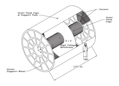
Figure 2.3: Schematic drawing of the STAR TPC [53].
