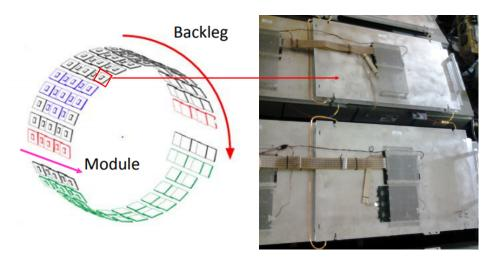
Figure 2.9: The left panel shows a cartoon of the modules arranged in backlegs around the STAR geometry, with the rest of the STAR detector removed (photo credit: [61]). The right panel shows a photo of some installed MTD trays on STAR taken by the author during the installation in Fall of 2013.
