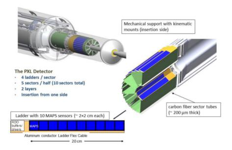
Figure 2.7: Schematic drawing of the PXL sub-detector of the HFT [57]. The PXL detector is arranged in sectors, with each sector containing ladders of ten PXL chips each. One ladder resides on the inner radius of the sector, and three are staggered to overlap on the outer radius of the sector. When the sectors are combined, an inner and outer layer of the PXL detector are formed, allowing for reconstruction of two hits for a single track much closer to the collision vertex than the TPC.
