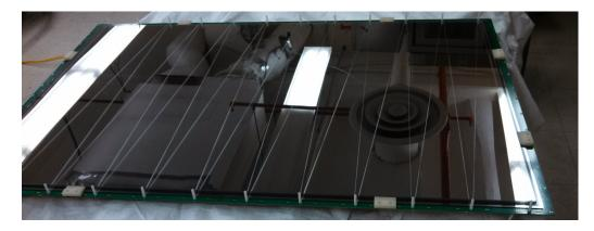
Figure 2.11: An MTD module with the top layer of honeycomb+PCB removed. The zig-zag pattern of nylon fibers separating the glass layers can be seen, as well as the carbon paint beneath the bottom-most glass layer.
