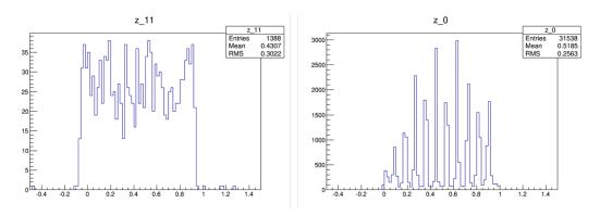
Figure 2.12: Plots of MTD noise rates (in Hz) as a function of percent of total length along strip. The left plot is from a "good" strip, with rates around 30-40Hz and no obvious noise pattern. The right plot is from a strip in a module with dirty nylon fibers, with extremely high noise rates ( $\sim 3000~{\rm Hz}$ ) and obvious periodicity of the noise consistent with the pattern of the nylon fibers.
