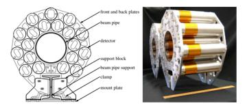
Figure 2.8: The left panel is schematic drawing of one of the upVPD asemblies, and the right panel is a photograph of both upVPD assemblies [60].
