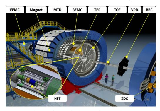
Figure 2.2: Schematic of the STAR detector, depicting the various detector subsystems at STAR. Of special interest to this thesis are the TPC, HFT, VPD, and MTD which are detailed in this chapter.
