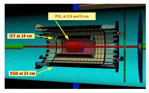
Figure 2.6: Schematic drawing of the Heavy Flavor Tracker.
