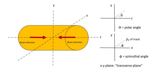
Figure 1.8: Cartoon illustrating a generic cylindrical detector with the axes labeled and relevant quantities noted.
