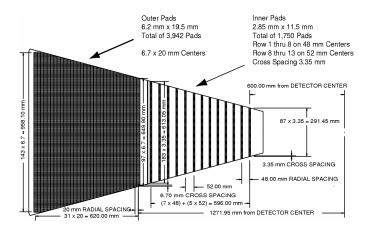
Figure 2.4: Schematic drawing of a STAR TPC sector, with the inner and outer sub-sectors differentiated. [53].
