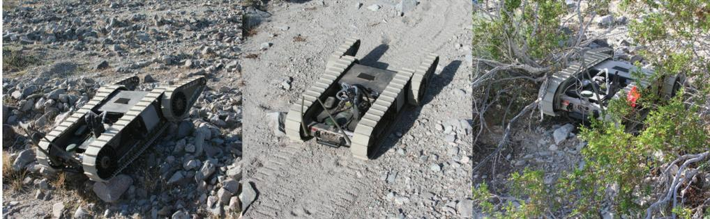
Figure 4.11: Deployed Packbot maneuvering through diverse terrain during the discharge test.
