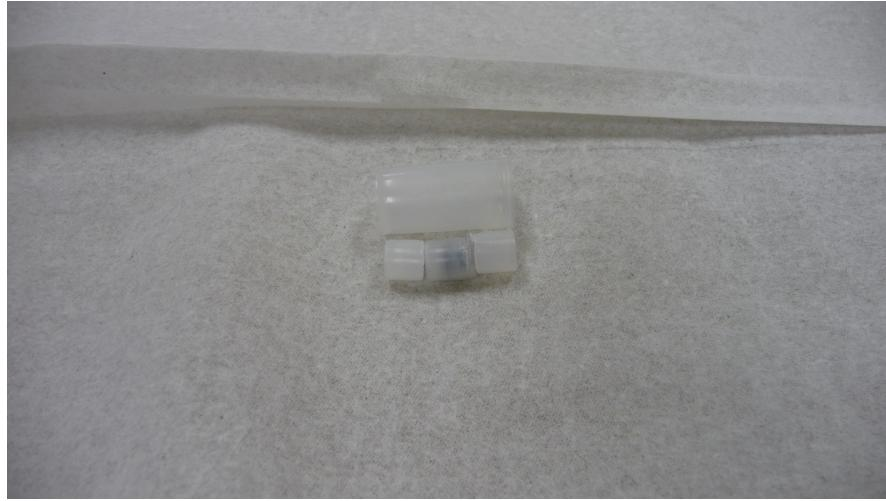
Figure 3.4: Small vial to be placed in the medium vial using halves of another small vial as spacers to center the sample.
