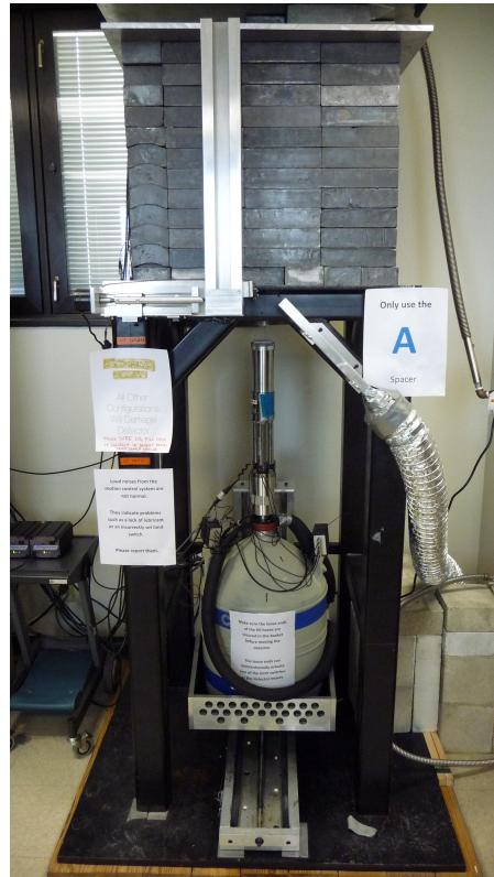
Figure 3.8: The HPGe detector setup.
