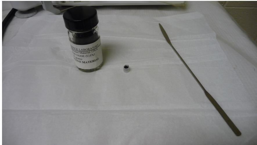
Figure 3.2: A small vial cut in half and filled with 0.1005 g of CRM 129-A.
