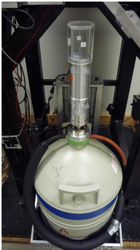
Figure 3.10: Position D on the detector is 9.0 cm from the face of the detector.
