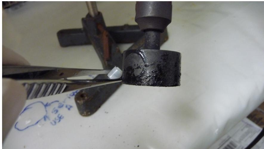
Figure 3.3: Heat sealing the small vial with CRM 129-A inside.
